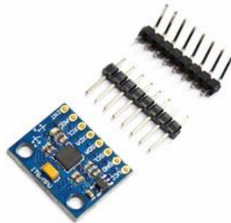
Gambar 3. modul sensor accelerometer MPU60X0 (sumber https://www.bazaargadgets.com/no/mpu9150-9-axis-akselerometer-sensor-modul-for-arduino-to-stil.html )
